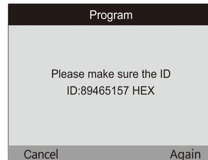
③ Manual ID creation: Select "Manual ID input (single)" to enter the ID input interface. Press the "Up/Down" keys to select the value you want to enter, then press "OK" to enter the corresponding value ("Backspace" can be used to delete the value entered, and **Dec↔Hex** can switch between input systems). Select "Enter" to complete the ID input and enter the ID confirmation interface.
